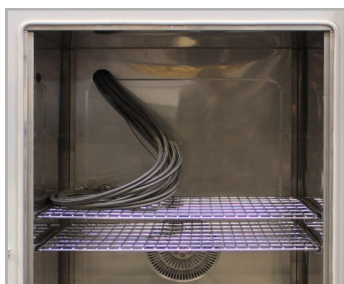
Access port—inside view
